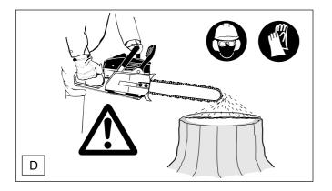
Never work with the chain saw withoute sufficient chain lubrication. Otherwise the service life of the chain and guide bar will be reduced.
